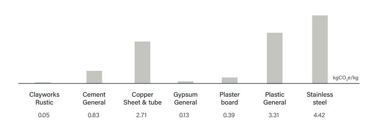
This graph demonstrates how clay plaster compares kilogram-for-kilogram with other materials. However, these values are not reflective of how we use materials in architecture and interiors. For example, we don't specify ceramics by the kg.
